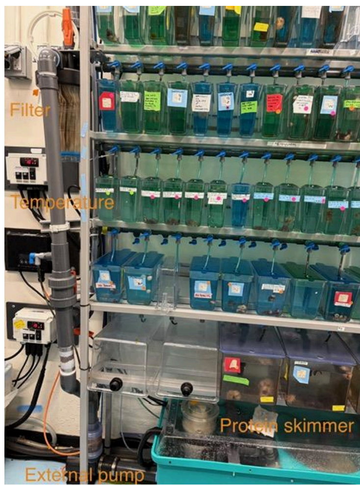
Figure 7. Pictured is an Aquaneering system with modifications for use with seawater and sea urchins. An external marine-grade Abyzz pump, a protein skimmer, and a system filter are the three major modifications. Note the different sizes of tanks used for husbandry of different lifestages.
